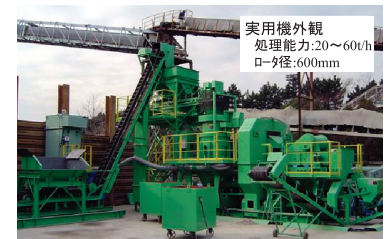
Photo 12 偏心ロータ式高品質再生骨材製造装置（実用機、処理能力=20t/h） Eccentric roter type machine for concrete recycle (Commercial machine, production capacity = 20t/h)
