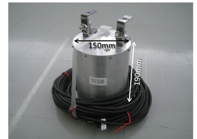
Photo 3 振動発電機 Vibration energy harvester
