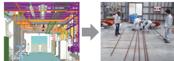
Factory production of pipes based on BIM 3-D data
