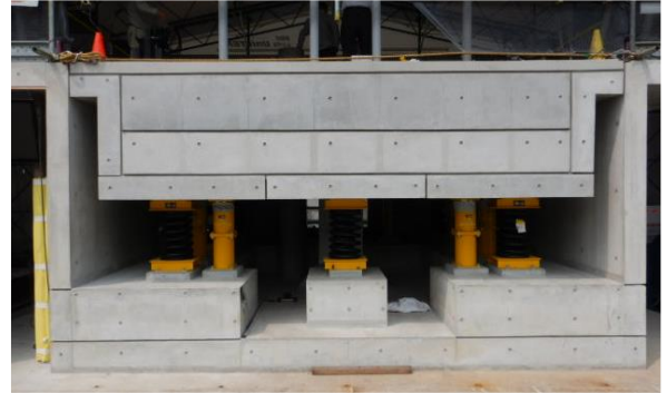
Photo 3 Mockup of anti-vibration floor
